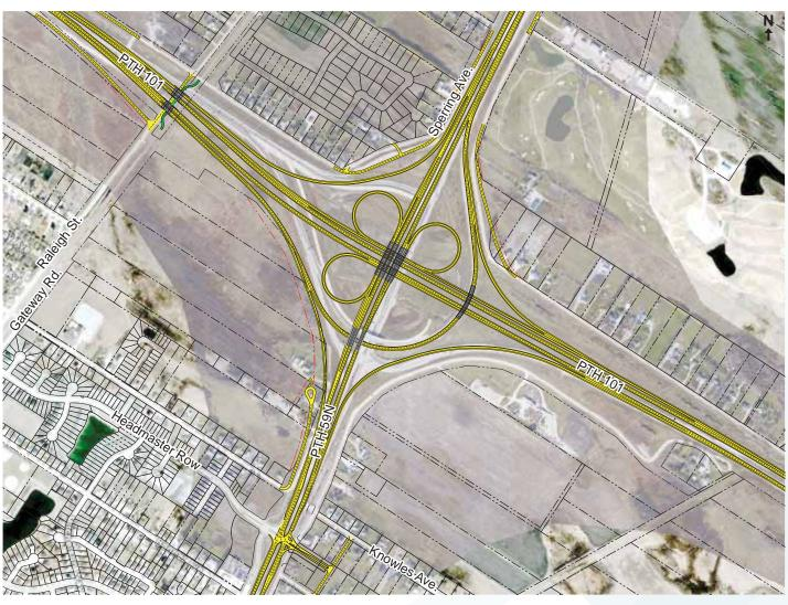
The interchange will accommodate future traffic by allowing the free flow of vehicles on both PTH 59N and PTH 101.
